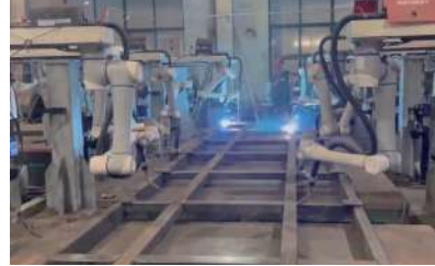
Carbon Steel Frame Welding
