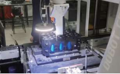
Energy Storage Battery Screw Locking
